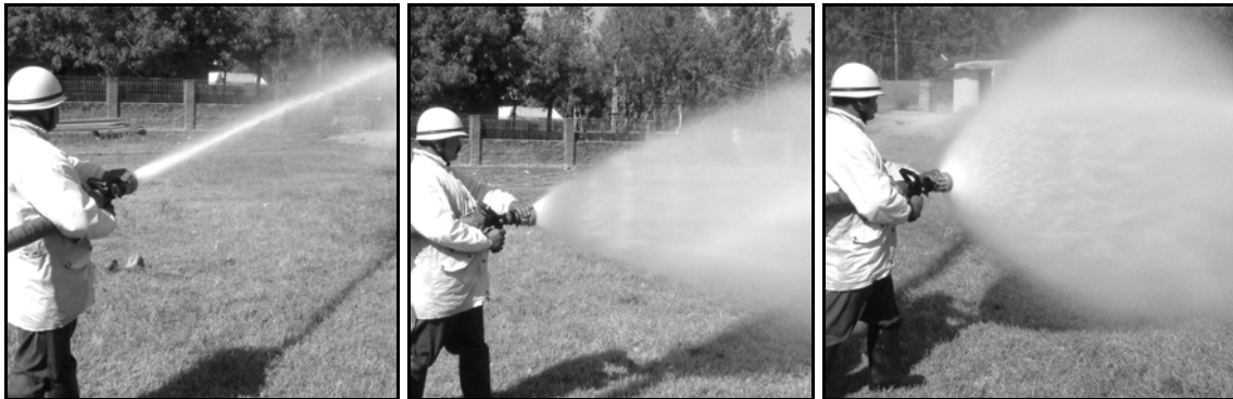
Combination (Jet/ Spray) nozzles are capable of giving different patterns (i) hollow jet for long range firefighting (ii) narrow fog for cooling or vapour dispersal & (iii) wide fog for radiant heat protection
