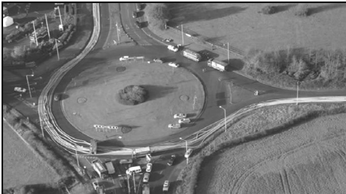
Fig. 2. A long hose relay system was used to supply water to the incident site
